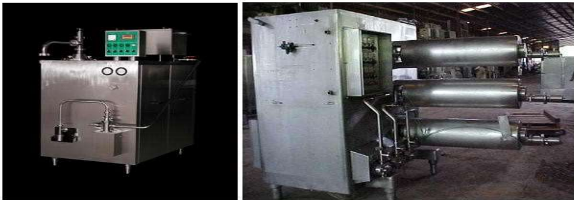
FIG-18.1 Continuous Ice Cream Freezer
